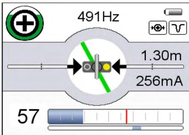
Along with the tracking signal, the new measurement screen provides a clear overview of all relevant information that can be useful in locating the cable or probe.
