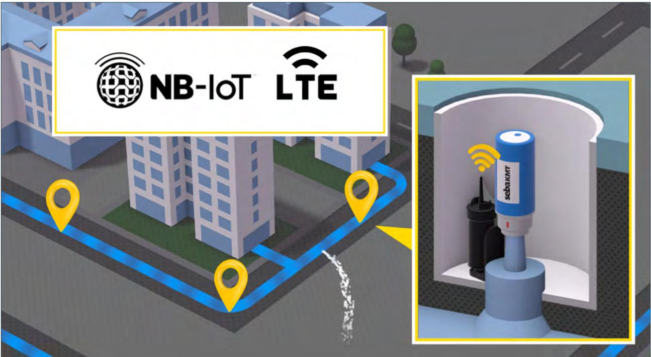
A measuring location contains two devices, the N-3 Noise Logger and the GT-3 NB-IoT transmitter, which is responsible for data transmission. The pair of measuring locations is supplied ready for use and pre-programmed in the factory.
