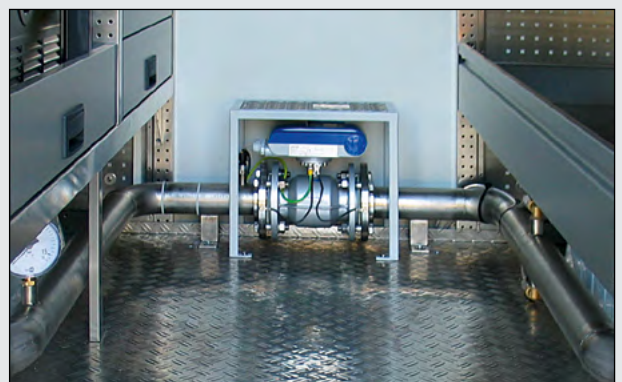
TDM 200 installed in a test van
