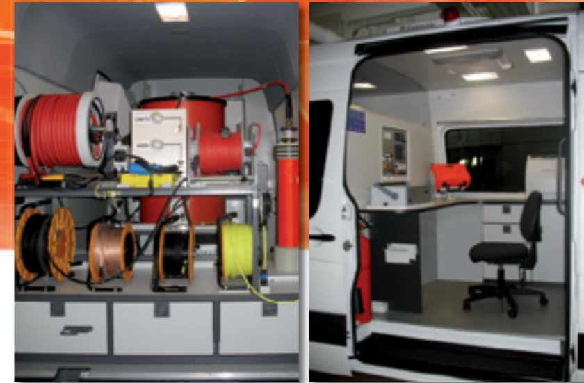
Test and diagnosis van with VLF CR-80 + OWTS M 60 and SPG 40
